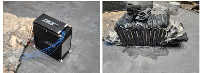
Fig. 13. Module condition after the thermal runaway propagation test: module exterior (left) and cell stack (right).
