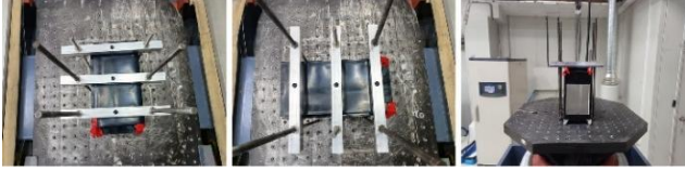
Fig. 10. Mechanical shock fixturing for X- (left), Y- (center), and Z-axis (right) orientations (30 g, 11 ms, both polarities each axis).
