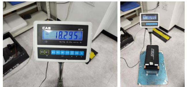
Fig. 2. Module mass measurement prior to energy density testing (Prototype #1, 18.295 kg): scale readout (left) and module on the platform scale (right).
