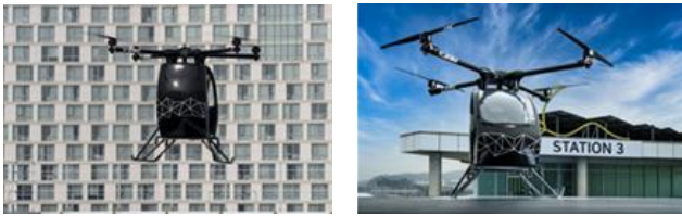
Fig. 14. V-Speeder X demonstrator powered by two series-connected modules (28S1P): hovering flight in an urban environment (left) and the aircraft at a vertiport (right).
